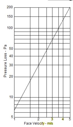
This graph enables the predicted pressure loss, or resistance of the louvre to be obtained at various airflow rates.
